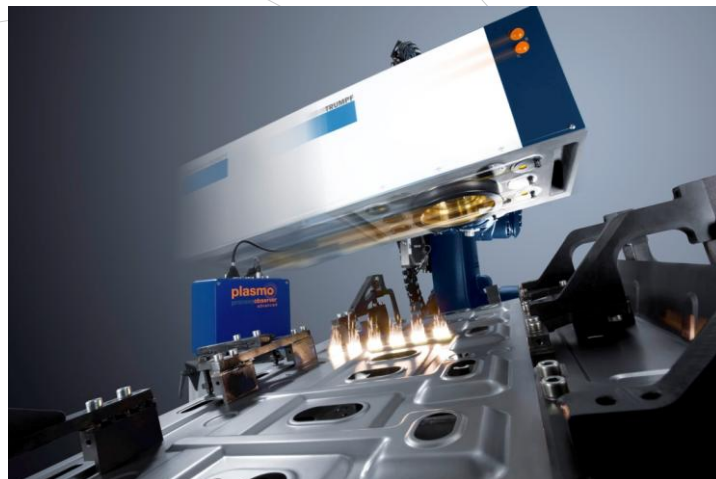
[Figure 5: Inline processobserver advanced monitoring in use with a Trumpf PFO 3D]
