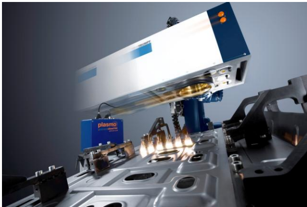
[Figure 2: Inline processobserver advanced monitoring used with Trumpf PFO 3D]
